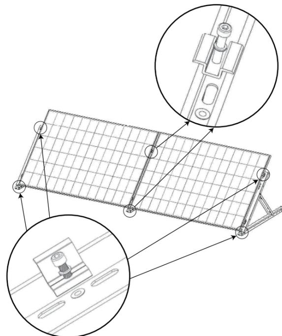
Step 4. Lock the Inter Clamps and End Clamps into the rivet nut.
