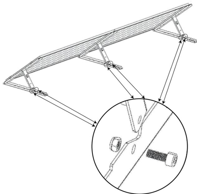
Step 3. Confirm the adjusted angle and lock the screws.
