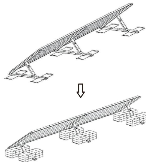
Step 5. Put the ballast plate in right position and place a heavy objects on the ballast plate. Finish.
