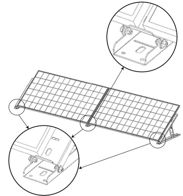
Step 2. Place the panels between two brackets as shown in the picture.
