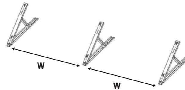
Step 1. Arrange the folding brackets with same angle at equal intervals.
